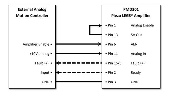
A high level on **Analog Enable** activates **Analog In**, easiest by connecting Pin 1 and 13 as shown in the figure above. Amplifier enable signal from the motion controller connects to **AEN** input and unparks motor on high level. Alternatively, connect the amplifier enable signal from the motion controller to **Analog Enable** and use a separate signal for park/unpark control to Pin 6.
