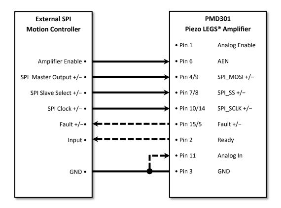
The SPI signals are AC-terminated with  $120\Omega$  in series with 1 nF capacitors. Single ended signals may be used if all inverted inputs are tied together and buffered with a 100nF capacitor.
