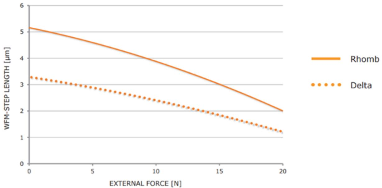
**Figure 1** Motor performance with waveform Rhomb (filled) and waveform Delta (dotted). Wfm-step length is the average distance the drive rod moves when the legs take one wfm-step (i.e. for one waveform cycle). Note: Standard deviation  $\sigma$  of  $0.5 \mu\text{m}$  should be taken into account. Typical values are given for  $20^\circ\text{C}$ .
