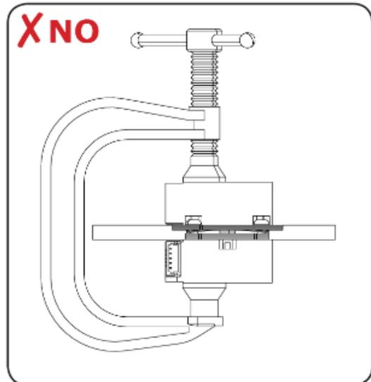
Always mount the drive rod using a mechanical adapter with flexible sheet metal extender so that transverse loads and torques on the drive rod are minimized. Never directly connect the drive rod and moving part in your application (for example when connecting the motor to a linear bearing). Mounting directly will introduce loads large enough for the drive rod to lose friction contact.
