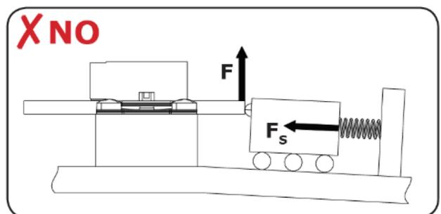
If acceptable, insert a thin piece of hard rubber between drive rod and stage block to minimize vibrations.
