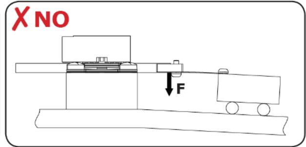
Misalignments in the drive plane are less critical but should be avoided. If the drive rod is aligned poorly there is risk for contact between drive rod and motor housing. Contact may impair function.
