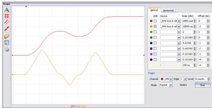
Note the controller treats the point where the velocity passes through zero as the end of one move, and the beginning of another move. It is allowed, however it will introduce some time delay.
