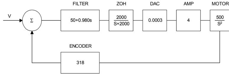
The open loop transfer function,  $A(s)$ , is the product of all the elements in the loop.
