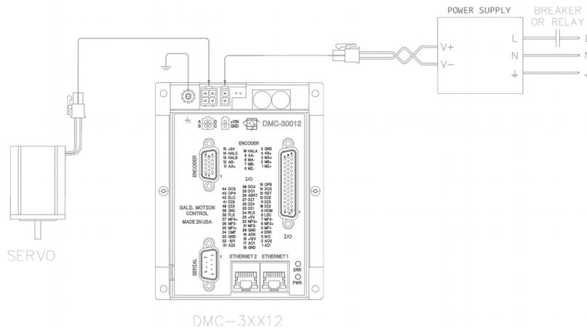
The green power light indicator should go on when power is applied.
