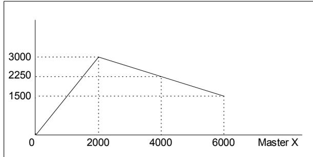
This disengages the slave axis at a specified master position. If the parameter is outside the master cycle, the stopping is instantaneous.
