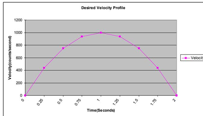
To accomplish this we need to calculate the desired velocities and change in positions. In this example we will assume a delta time of ¼ of a second, which is 256 samples (1024 samples = 1 second with the default TM of 1000).
