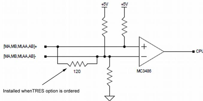
**Single-Ended Encoders:** Single-ended encoders will not operate correctly with the termination resistors installed. If a combination of differential encoder inputs with termination resistors and single ended encoders is required on the same controller, contact Galil directly.
